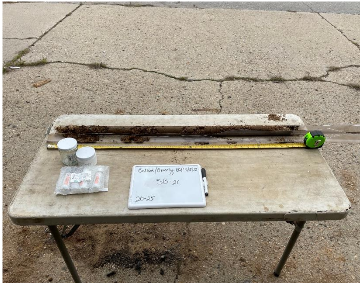
Photo 2: View of soil from SB-21 from 20-25 feet below grade surface, facing east.
