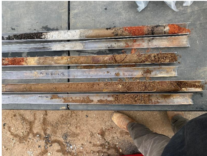
Photo 2: View of waste characterization soil boring cores, facing east.
