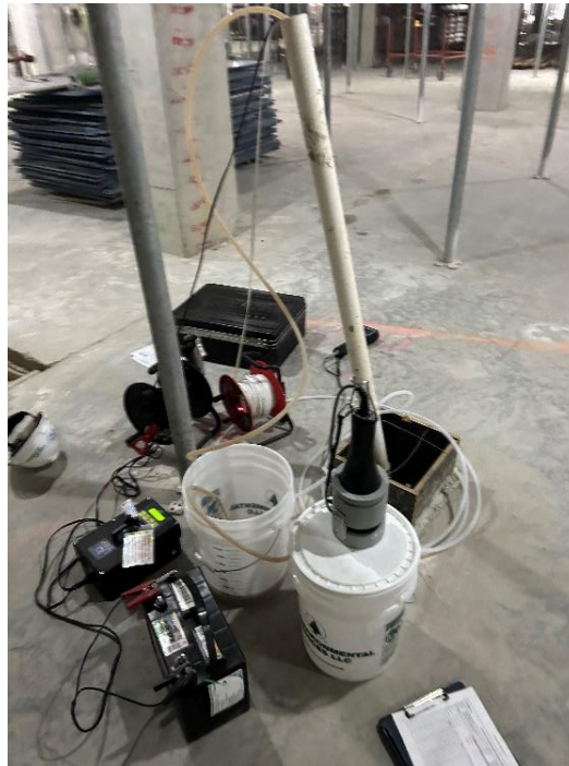
Photo 2: View of groundwater sampling setup at monitoring well PR-MW-01, facing north.
