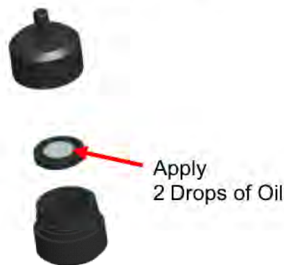
Figure 4-4: Apply 2 Drops of Oil to Impactor Plate
