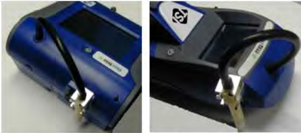
Figure 2-8: Installing Dorr-Oliver Cyclone
