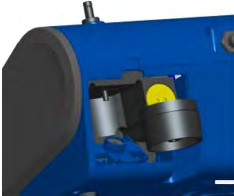
Figure 4-8: Remove 37-mm Filter Cassette
