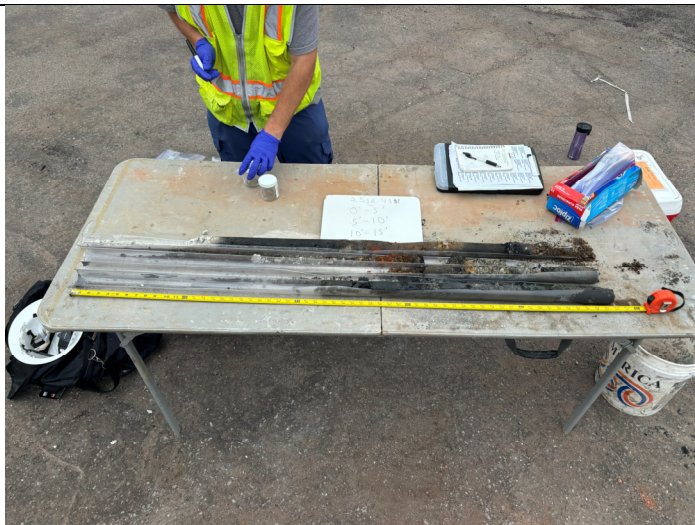
Photo 4: View of 25SB-4S2 soil boring from 0 to 15 feet.
