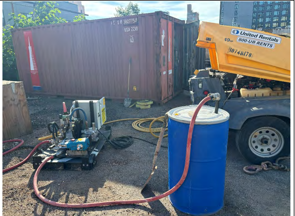
Photo 1: View of Atmos foam sprayer and compressor setup prior to intrusive work looking northeast
