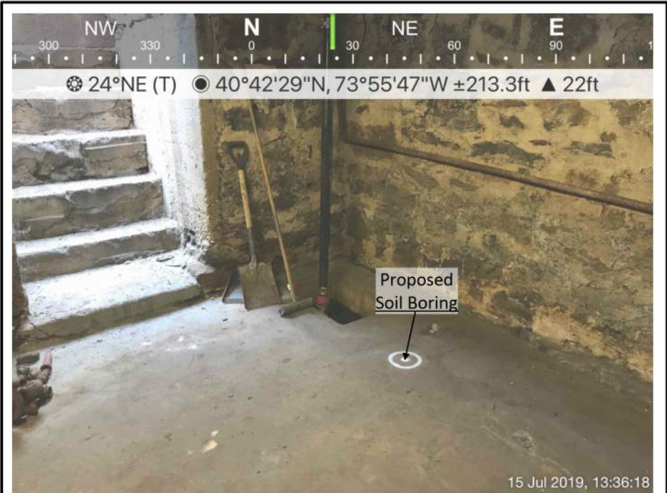
Northeast-looking site photo showing proposed soil boring and site features. No utility pipelines were detected within the image area. All Radiofrequency (RF) responses were low and constant, and GPR data were not indicative of utilities.
