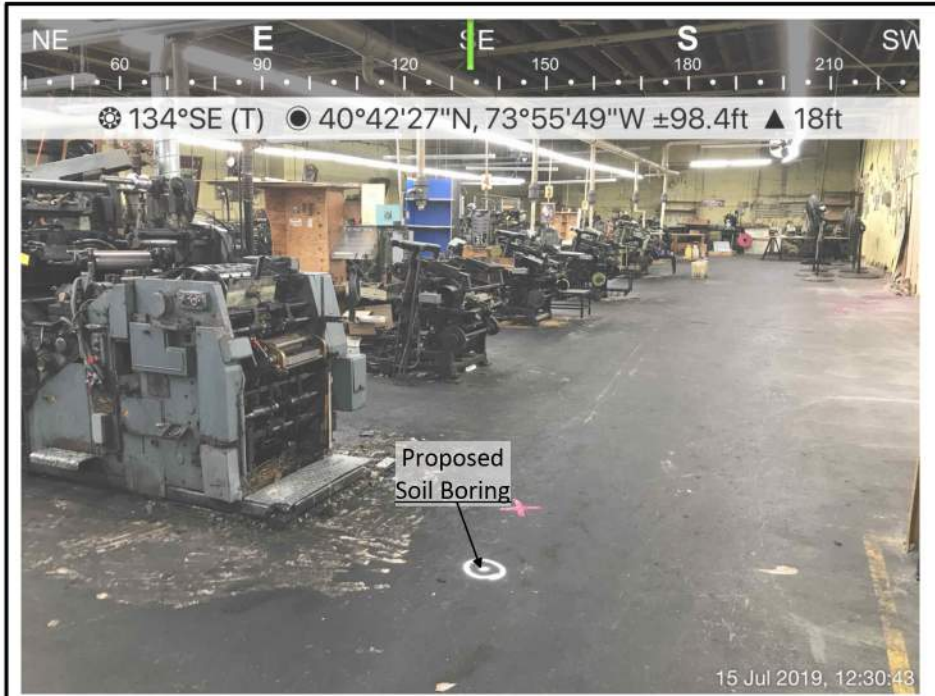
Southeast-looking site photo showing a proposed soil boring, detected spot anomaly (magenta "X"). No other utilities were detected in the image area. GPR data were excellent and all RF responses were low and constant.
