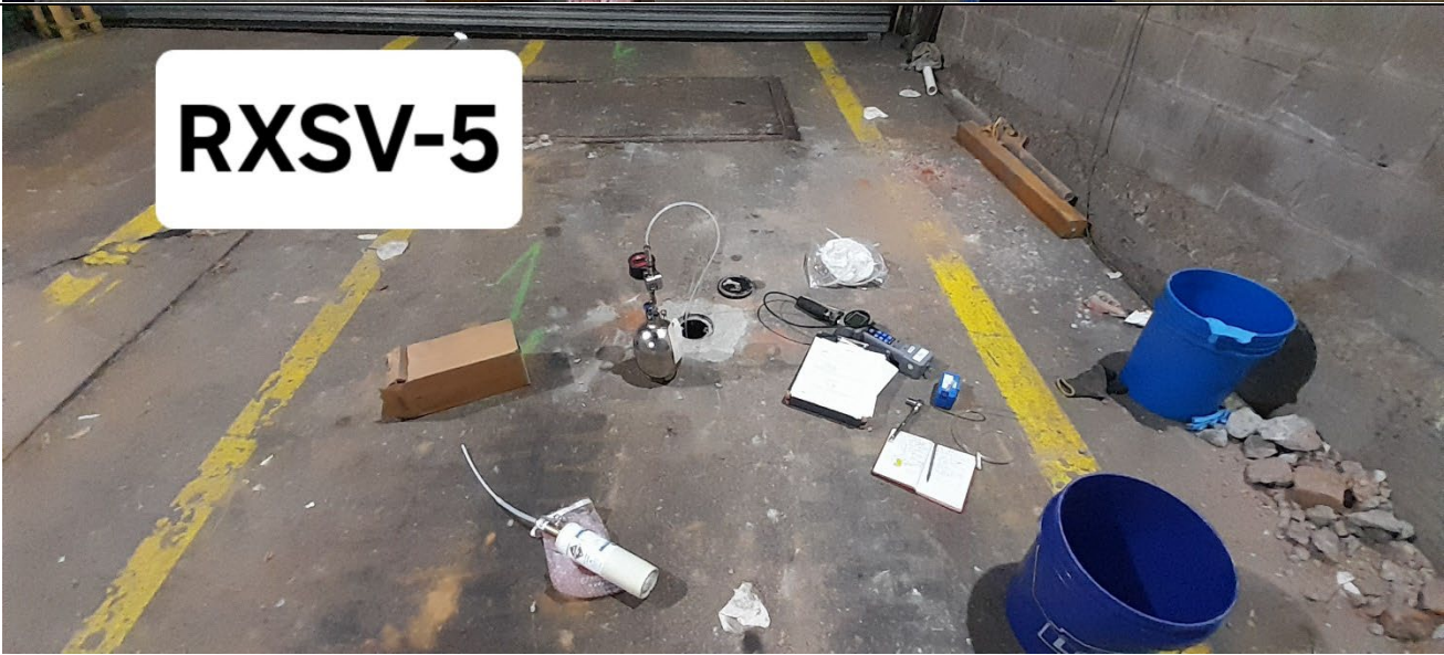
Photo 4: Soil vapor collection at RXSV-5
