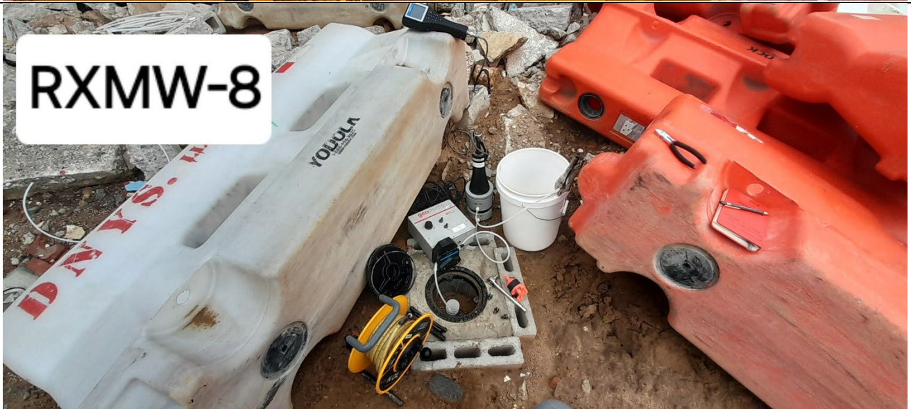
Photo 2: Groundwater sample collection at RXMW-8.
