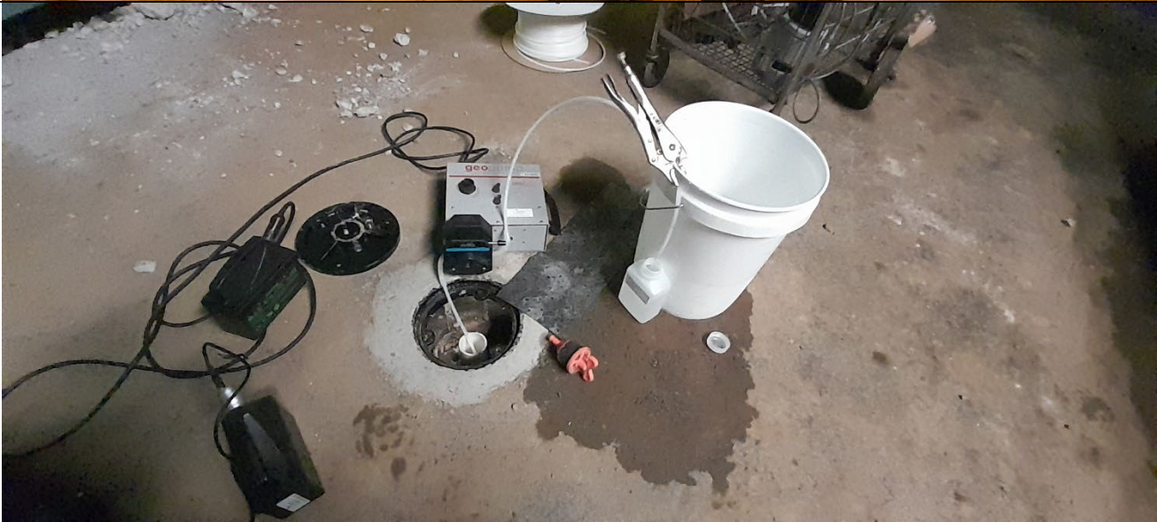
Photo 2: Groundwater sample collection at RXMW-7.
