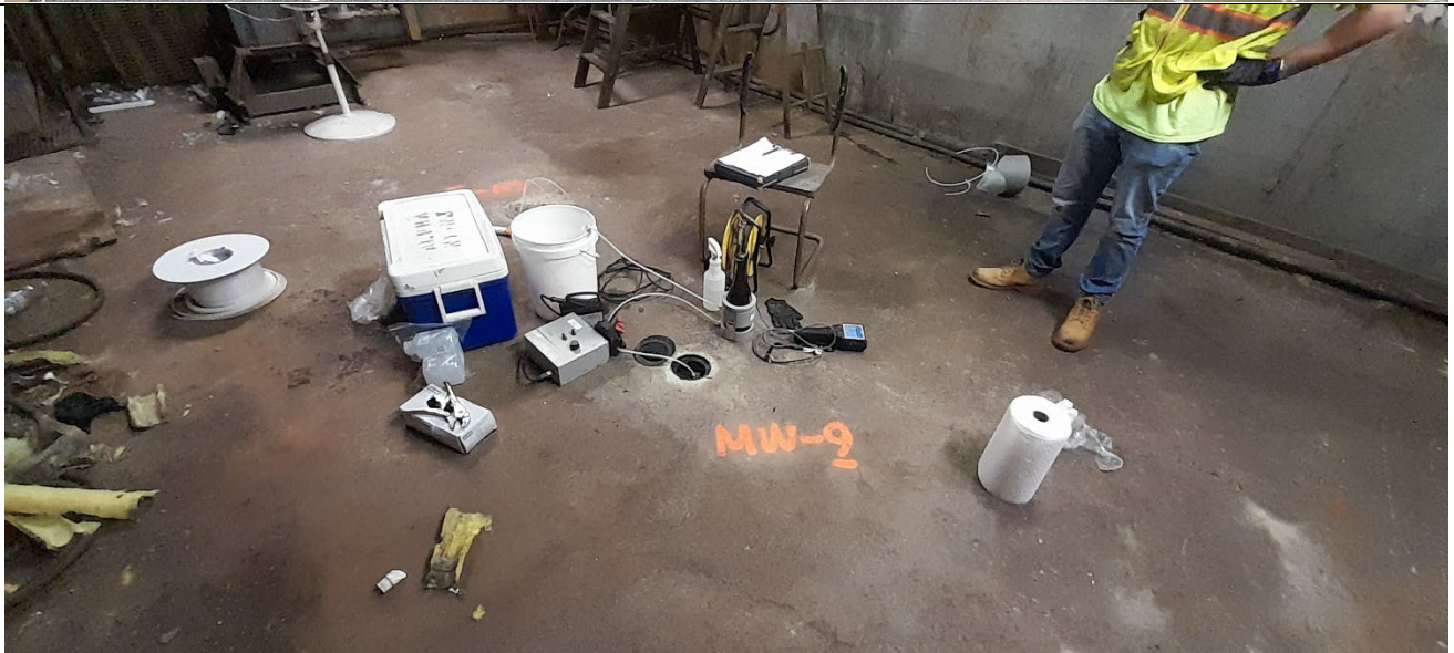
Photo 2: Groundwater sample collection at RXMW-9.
