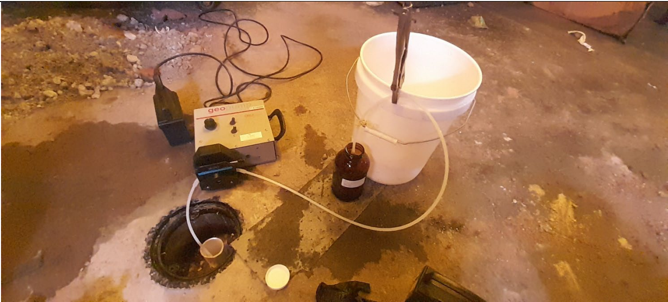
Photo 1: Groundwater sample collection at RXMW-11.
