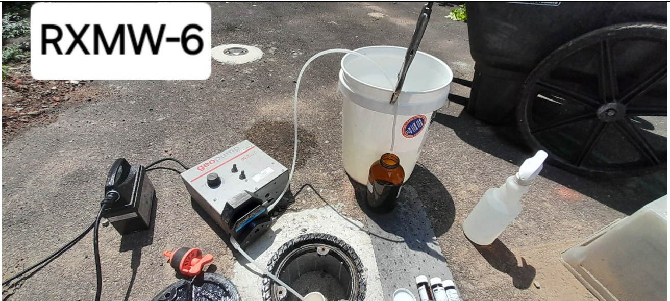
Photo 2: Groundwater sample collection at RXMW-6.
