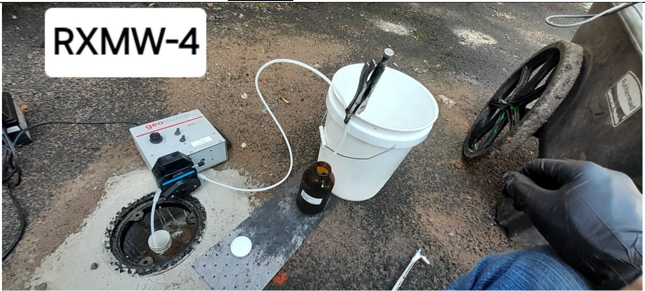
Photo 1: Groundwater sample collection at RXMW-4.
