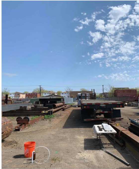
3. Performing groundwater sampling
