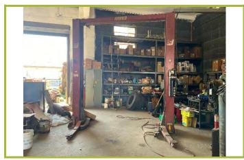
**Photo #13:** View of aboveground hydraulic lift within warehouse portion of the building.
