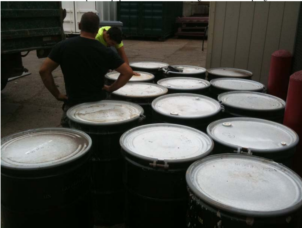
Photo 12- Drums of investigation derived waste (IDW) stored at the property and awaiting disposal, pending laboratory analytical results.
