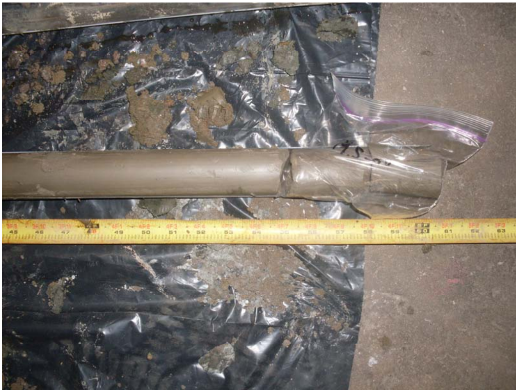
Photo 8- Varying degrees of saturation were noted below the groundwater table due to the fractions of clay present in the soil column. Note the stiff clay present in the 15-20' soil core.
