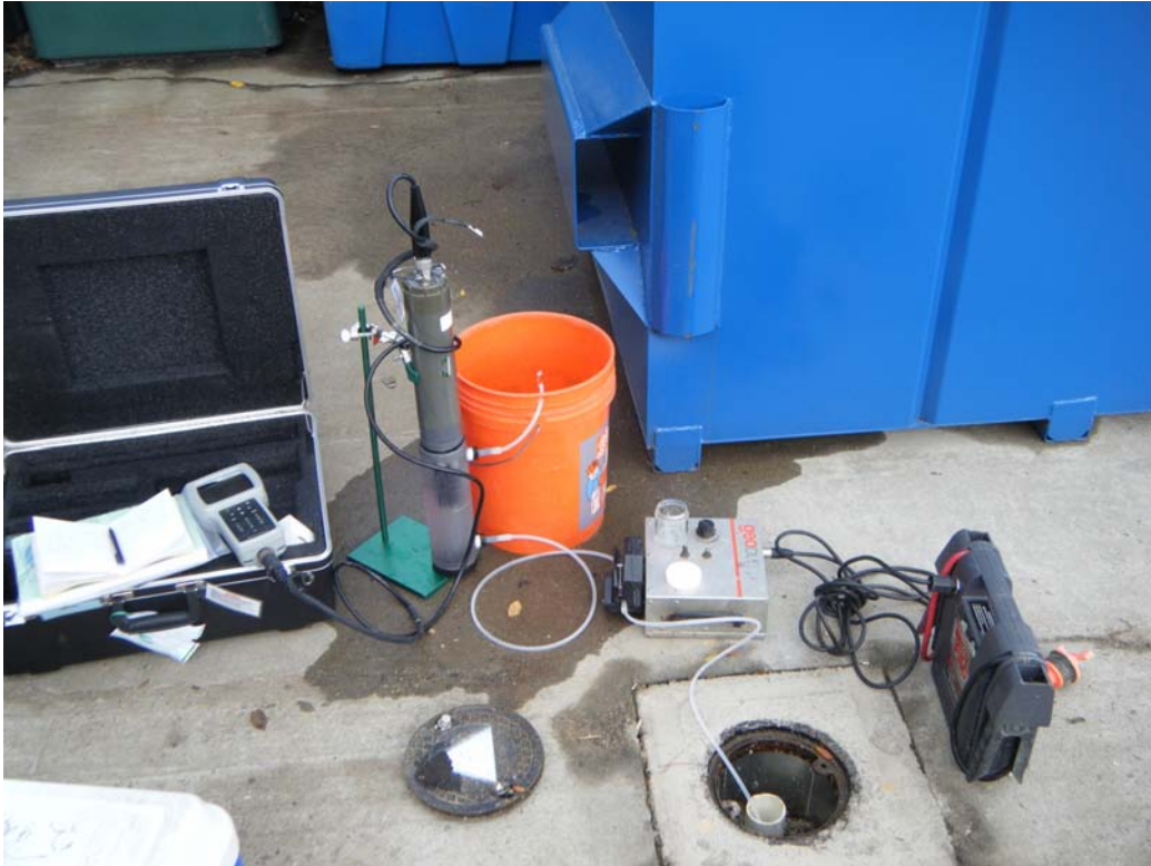
Photo 11- Example of equipment used for low flow groundwater sampling.
