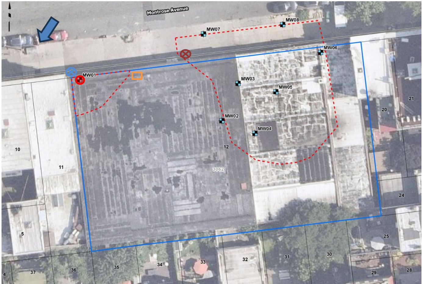
Figure 1: Monitoring Well Location Map
