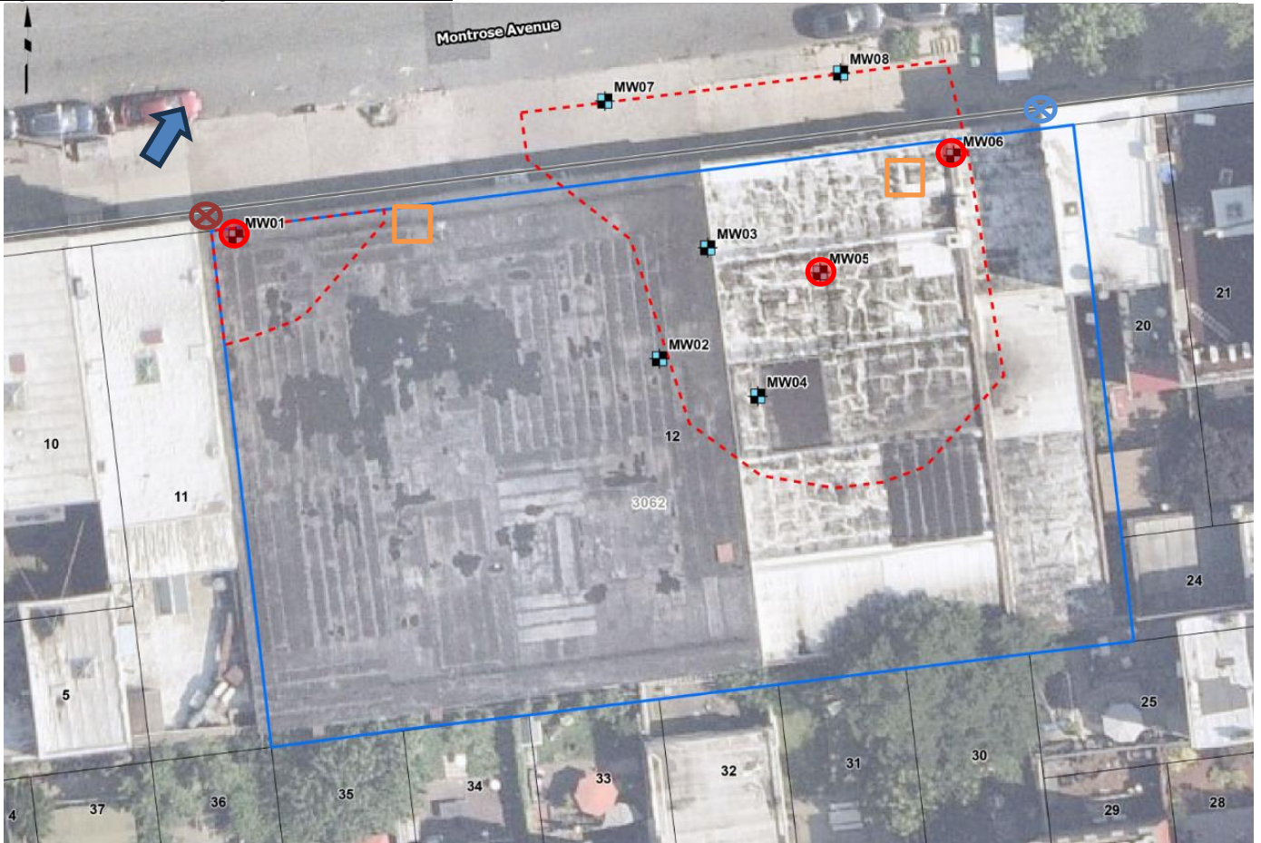
Figure 1: Monitoring Well Location Map
