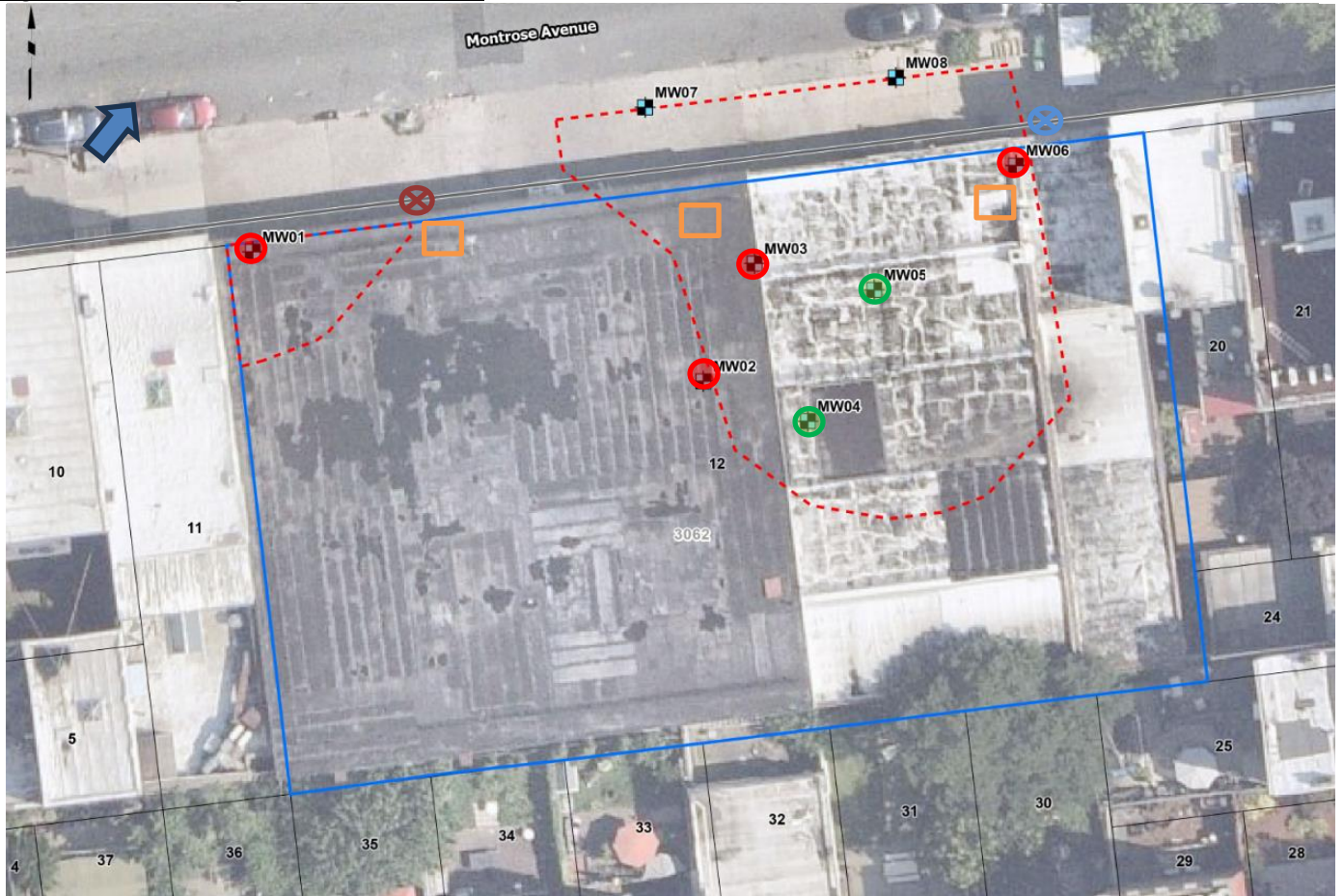
Figure 1: Monitoring Well Location Map
