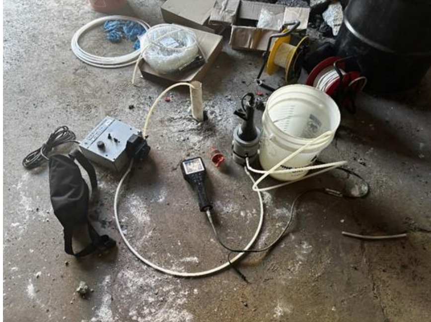
Photo 1: View of low-flow groundwater sampling setup at monitoring well MW06 (facing northeast).
