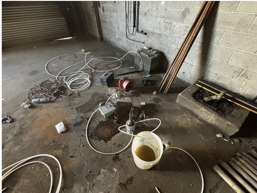
Photo 2: View of low-flow groundwater sampling setup at monitoring well MW03 (facing northeast).
