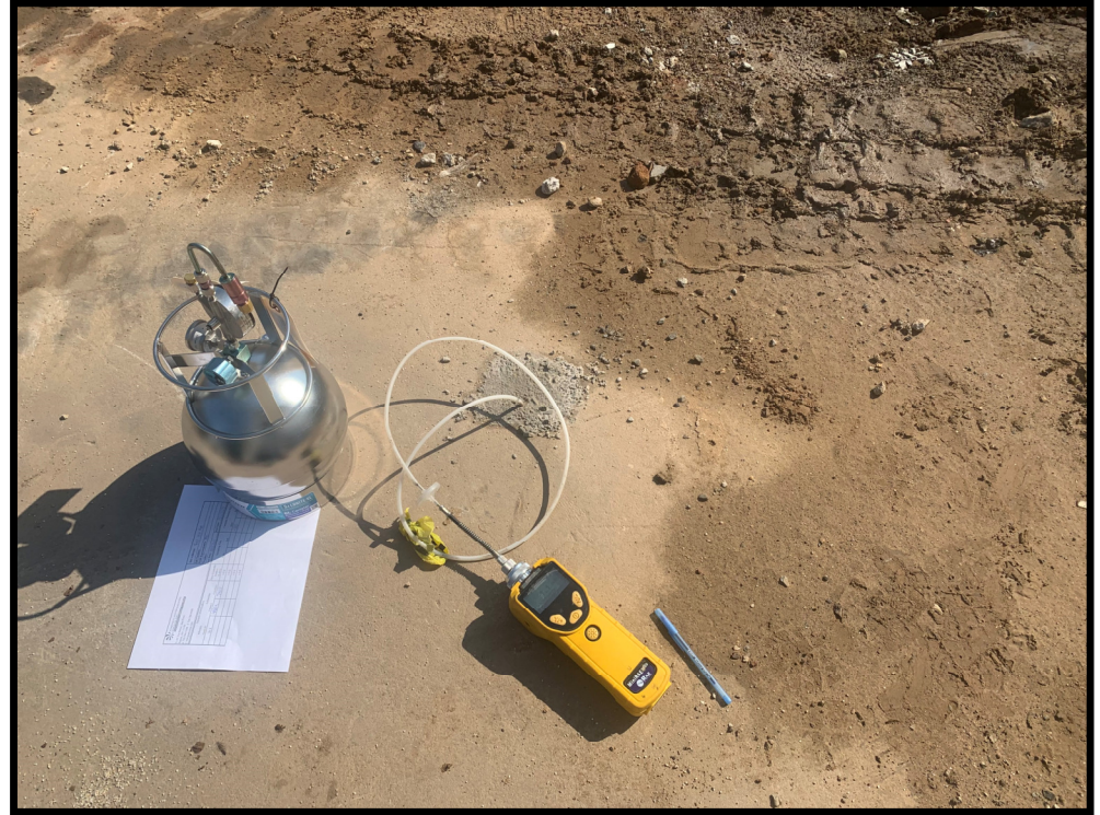
View of soil vapor point SV-2 being purged with a PID.
