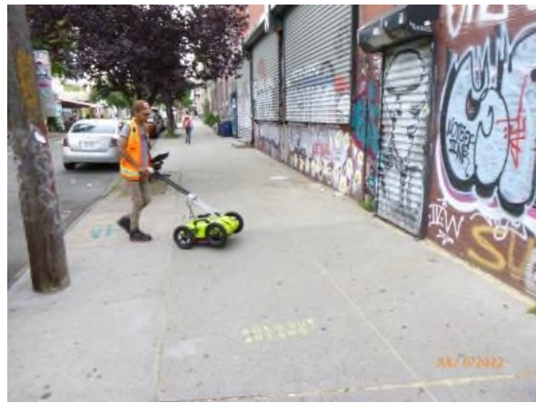
2. GPR survey in progress. UST vent pipe visible against building wall. Photographer facing northeast.
