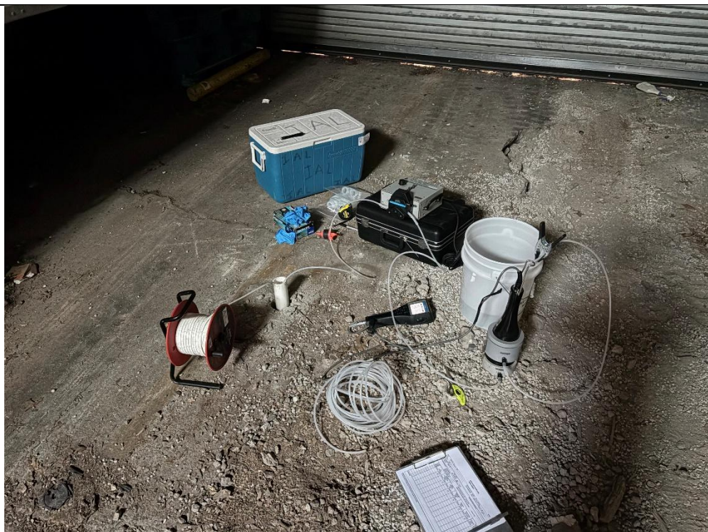
Photo 1: View of low-flow groundwater sampling at MW-4.
