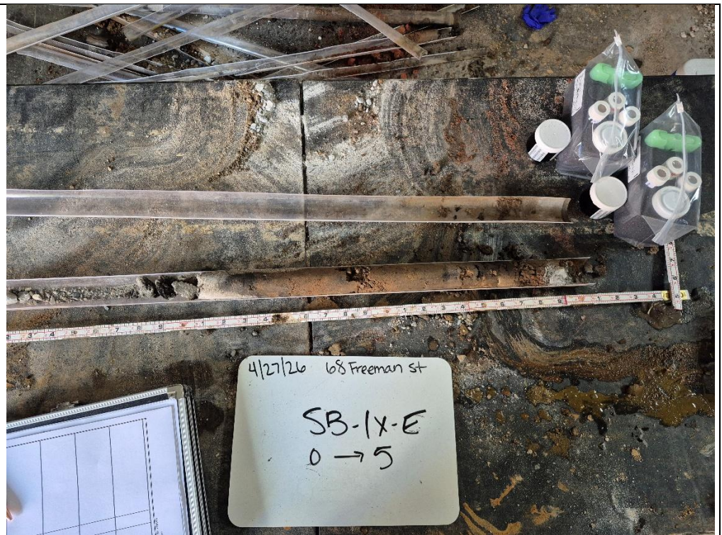
Photo 1: View of soil logging and sampling.
