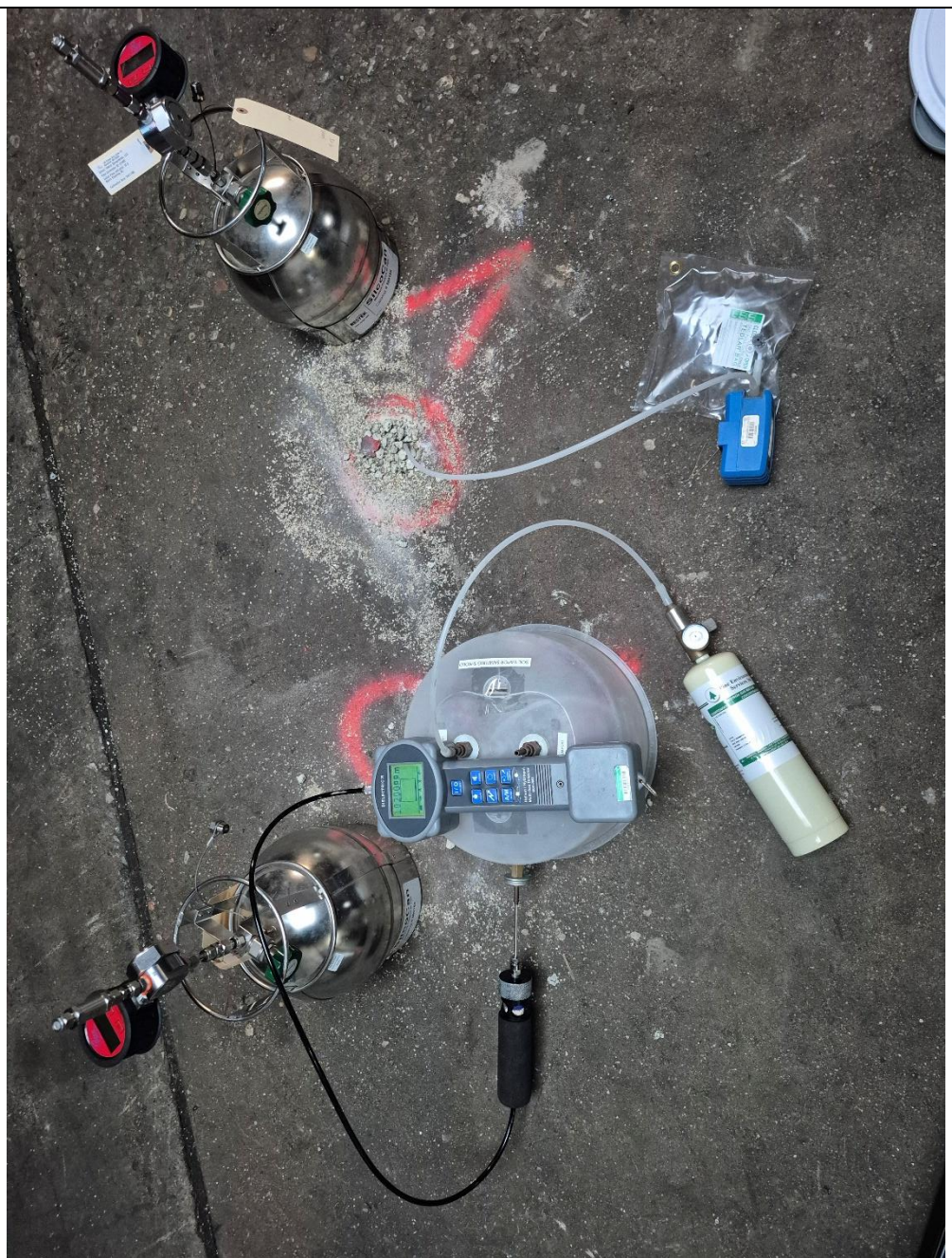
Photo 1: View of helium leak test and purging at SV-6 and DUP-1.
