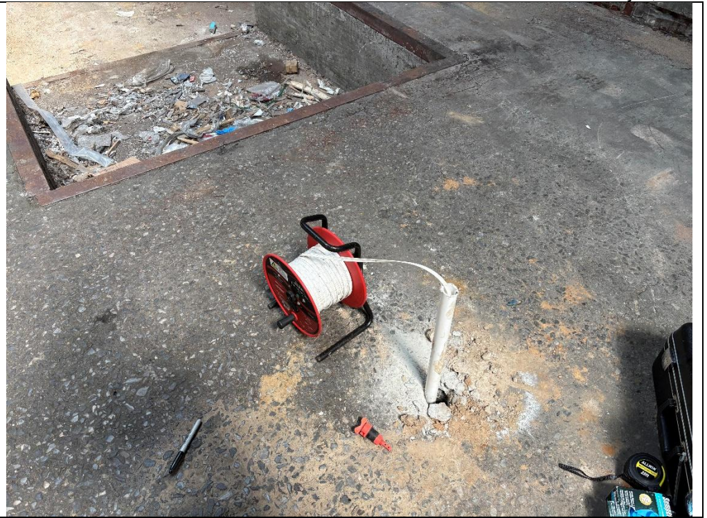
Photo 3: View of measuring groundwater depth in MW-3.
