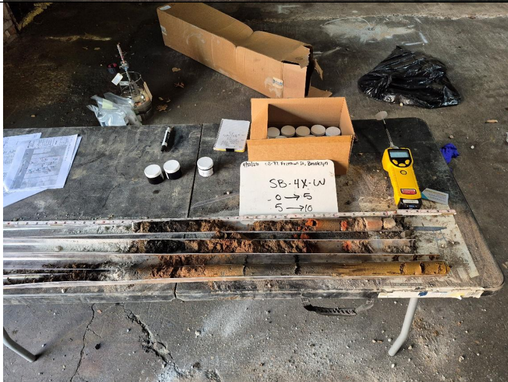
Photo 4: Representative view of soil boring cores and soil sampling.
