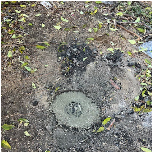
23. Groundwater Monitoring Well
