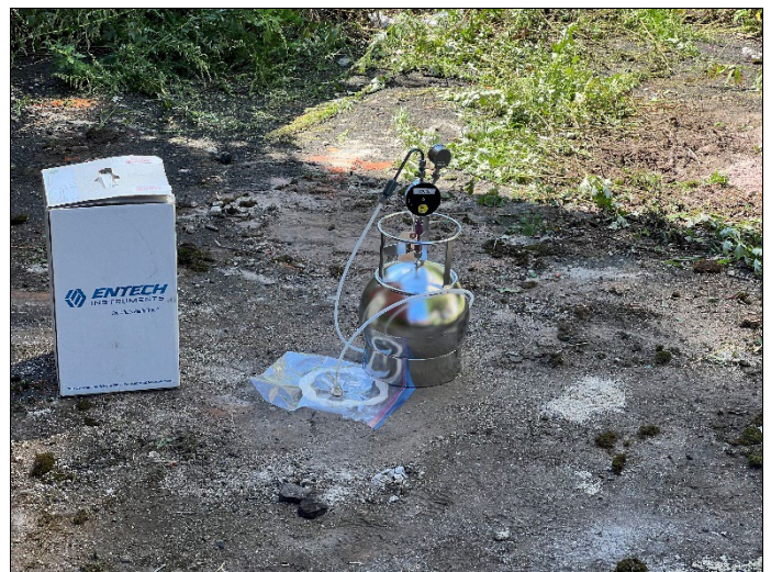
12. Soil Vapor Sample Collection (September 2024)
