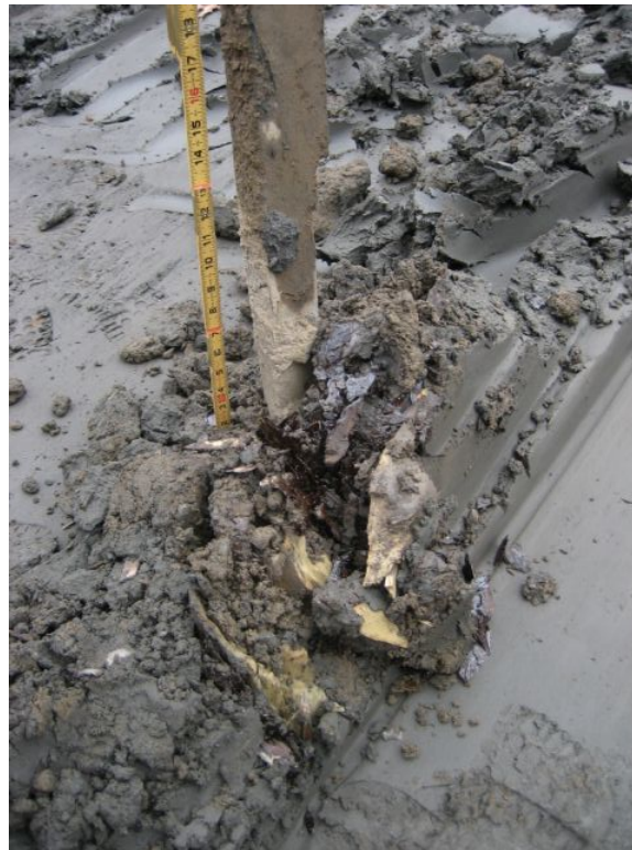
Figure 2. Wood stake indicates approximate location where refusal was encountered. Note the timber pile that is in the same area.
