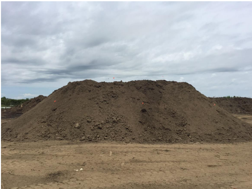
Photograph 2: View of manufactured organic topsoil stockpile; orange flags mark grab sampling locations (facing south)
