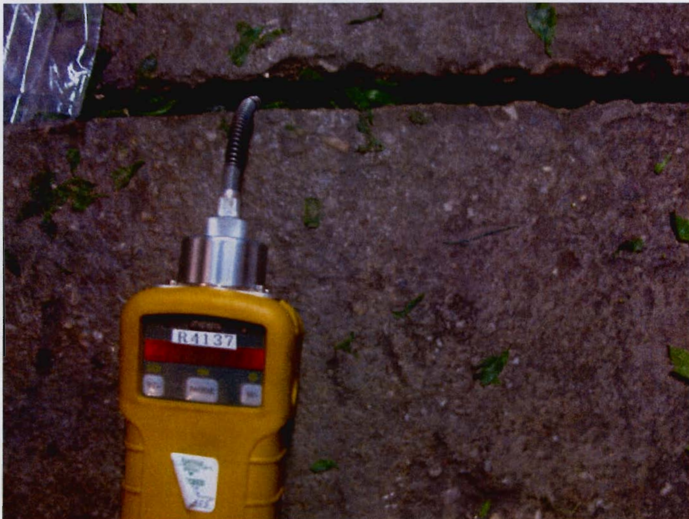
Photoionization detector monitoring in floor crack by florist work area during EMTEQUE's site inspection.
