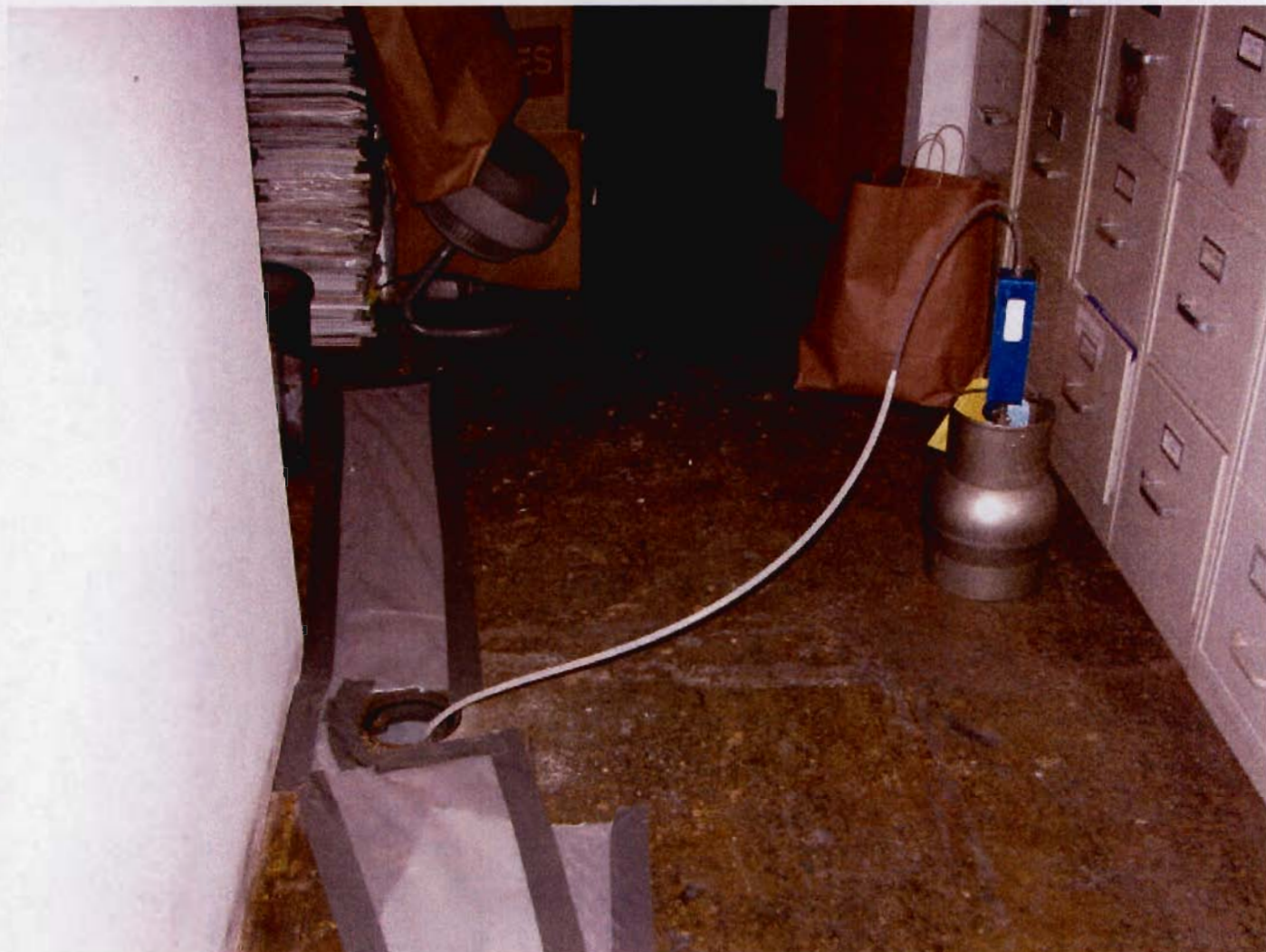
TRC Environmental Phase I air sample from SG-2. This is the typical TRC soil gas monitoring point sample set-up. Note polyethylene sheeting and duct tape utilized to seal crack running through the area of the soil gas point.
