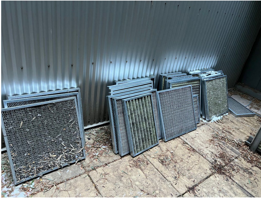
Photograph 5. Used and Replaced GSF-C-1 Air Filters (January 24, 2025).
