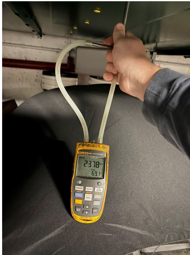
Photograph 6. Manometer and Pitot Tube Monitoring Equipment Measuring Air Velocity in GSF-C-1 Air Duct (January 24, 2025).
