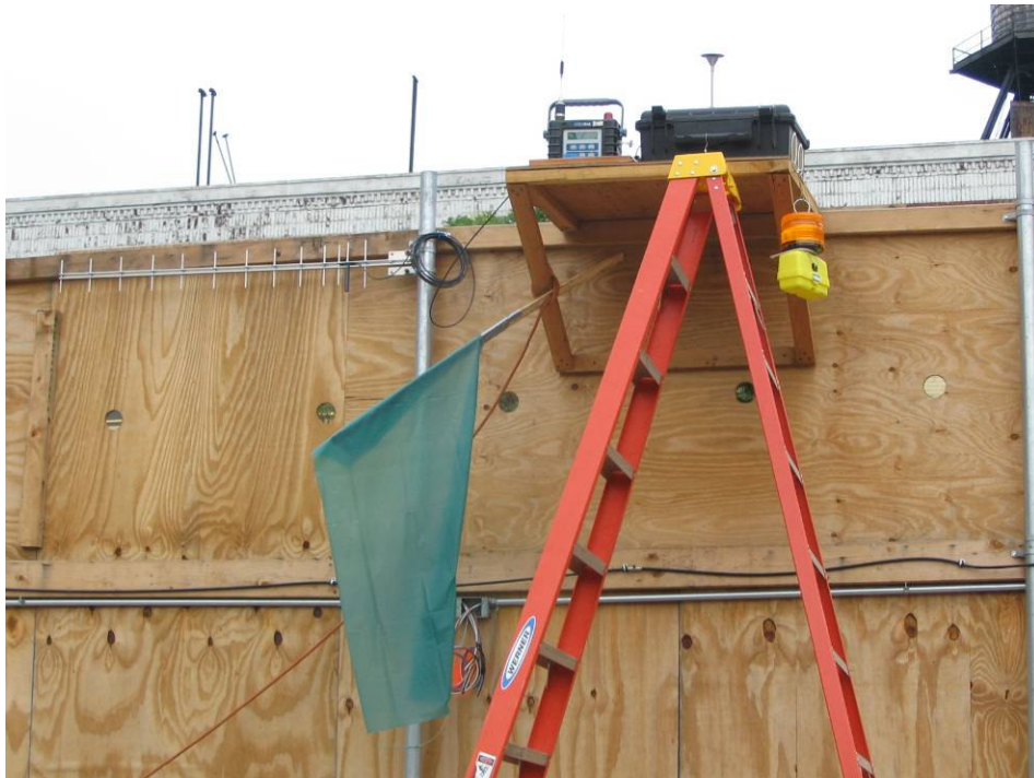
Photograph No. 16: View of typical Air Monitoring Station and telemetry with colored flag indicating current action level (green; VOCs < 3.7 ppm and particulates < 113 ug/m 3 ).
