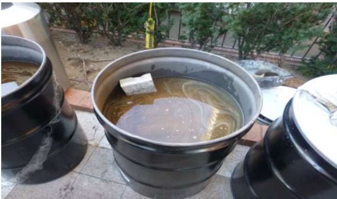
Photograph 2: View of impacted pavers in degreasing solution.
