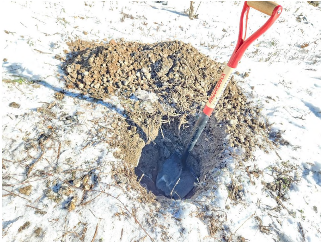
Photo 12: 2 ft. Test Pit to confirm RCA depth (January 17, 2024)
