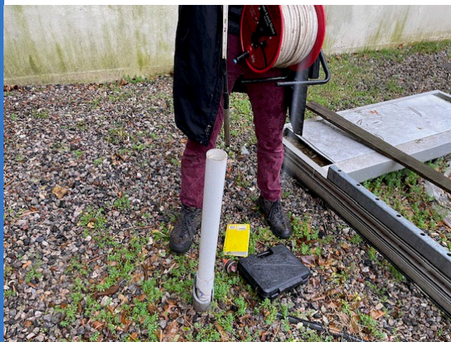
Photo 4: Well M-10C remains intact with repaired casing.
