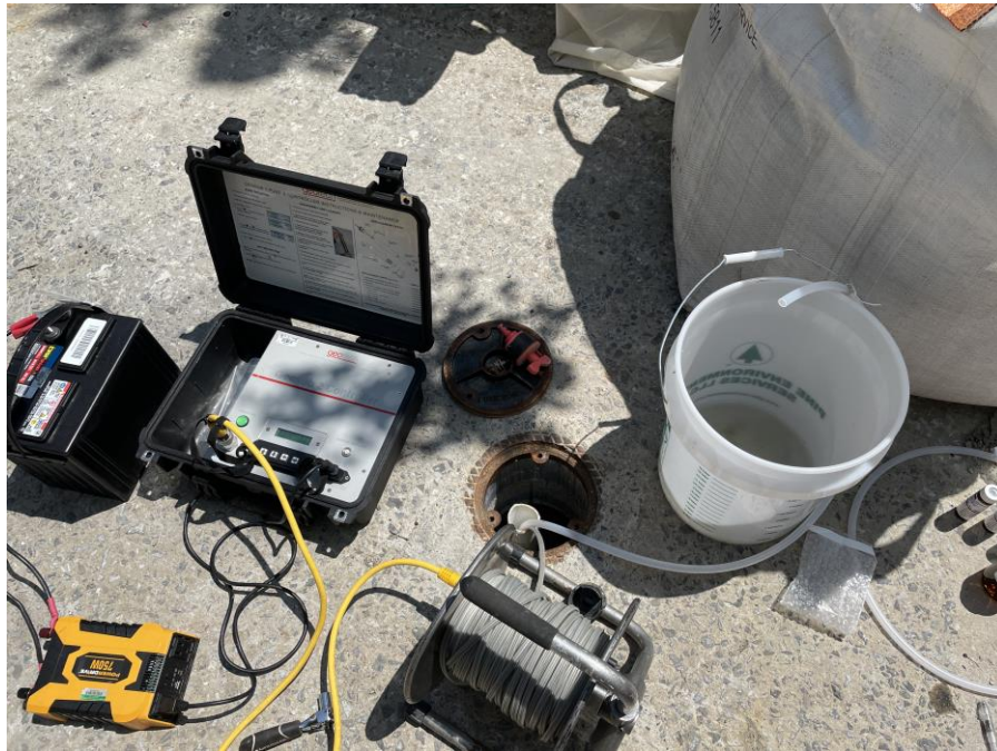
Photo 1: View of MW12 groundwater sample collection setup (facing south).
