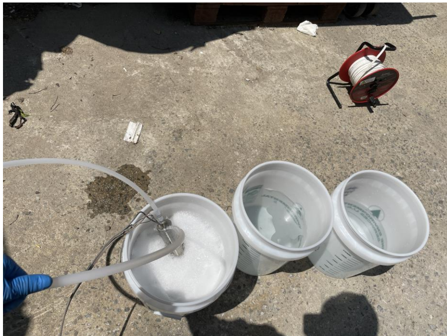
Photo 2: View of pump decontamination between use (facing west).
