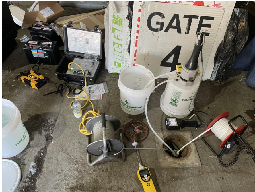
Photo 1: View of Langan purging groundwater from monitoring well MW-11 (facing southwest).
