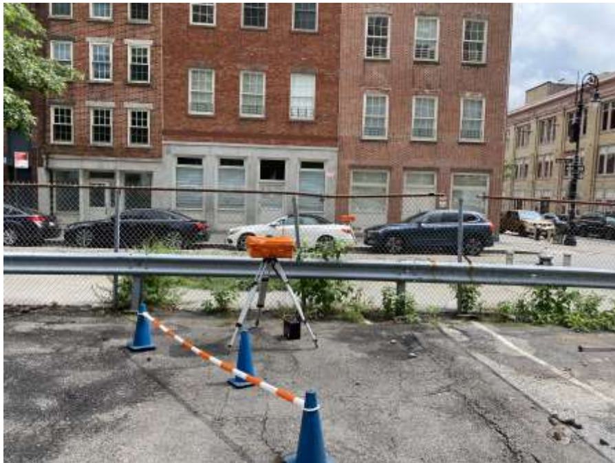
Photo 2: Perimeter CAMP station WZ-1 and off-site CAMP station PM-1 along Water Street during the drilling of boring SB28 (facing east).
