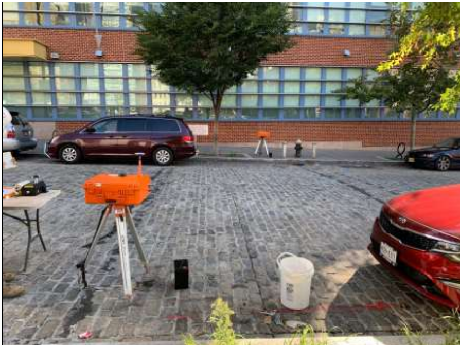
Photo 2: Perimeter CAMP station WZ-1 and off-site CAMP station PM-5 along Peck Slip during the attempted drilling of boring SB34 (facing northeast)
