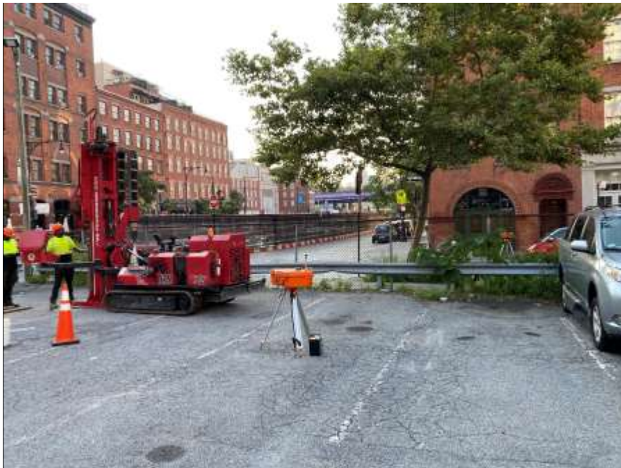
Photo 2: Perimeter CAMP station WZ-1 and off-site CAMP station PM-6 along Water Street during the drilling of boring SB35 (facing southeast)
