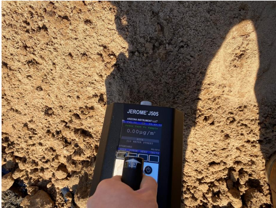
Photo 5: View of Langan screening excavated soil/fill from test pit TP01 using a Jerome® J505 mercury analyzer.
