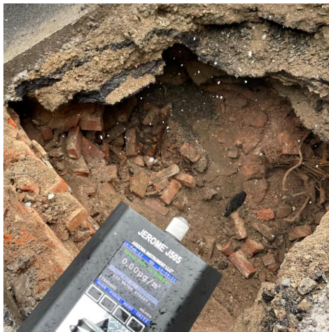
Photo 2: View of Langan screening test pit TP04 using a Jerome® J505 mercury analyzer.
