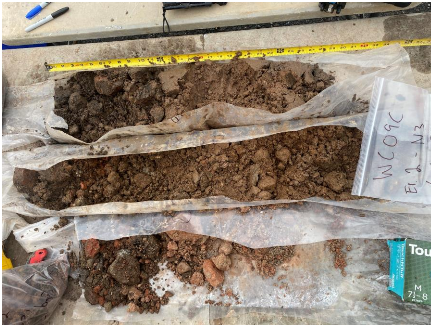
Photo 2: View of soil/fill recovered from waste characterization soil boring WC09C.
