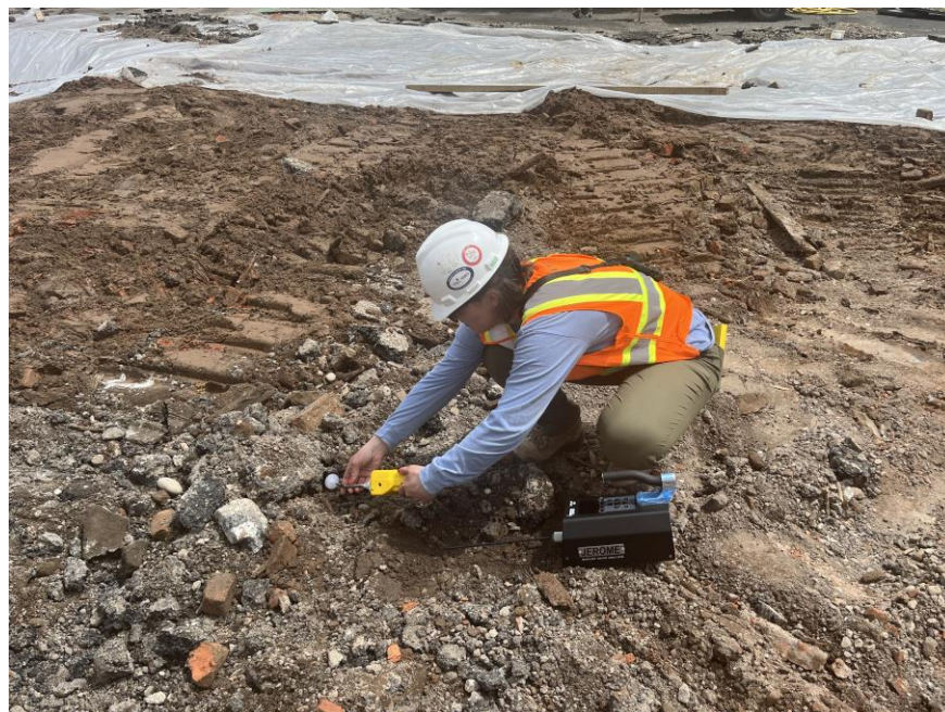
Photo 4: View of Langan screening exposed soil/fill using a Jerome® J505 mercury vapor analyzer and a PID (facing south).
