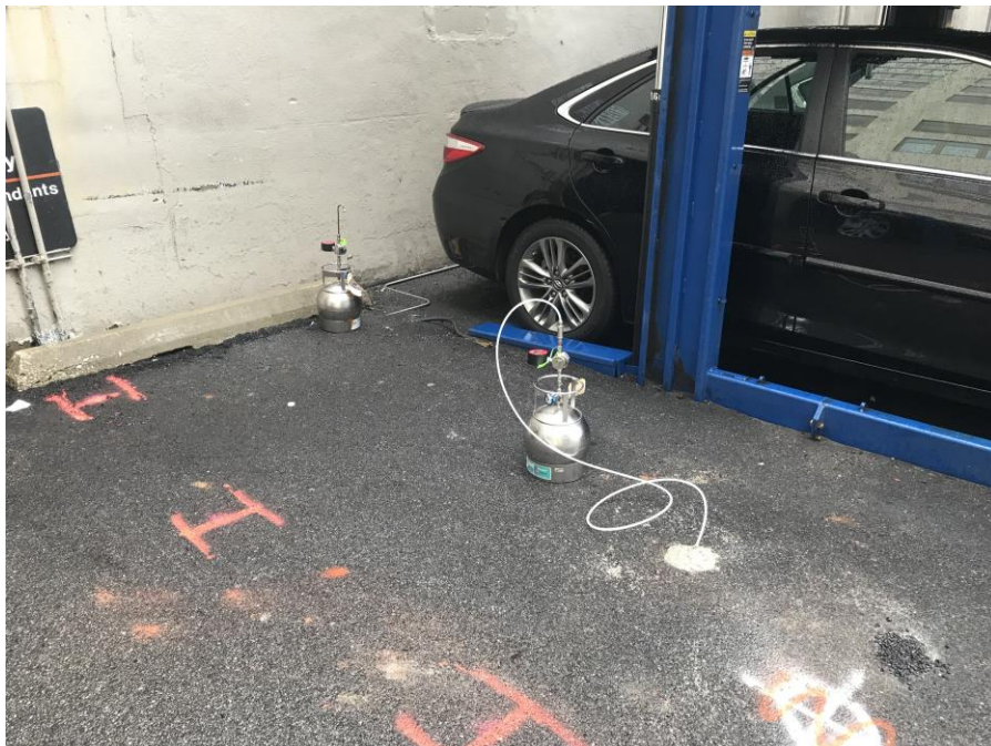
Photo 8, 4/25/2018: View of soil vapor sampling and ambient air sampling, facing southwest.
