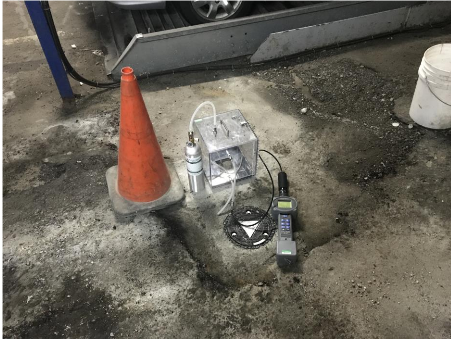
Photo 7, 4/25/2018: View of helium test being conducted at a soil vapor point.
