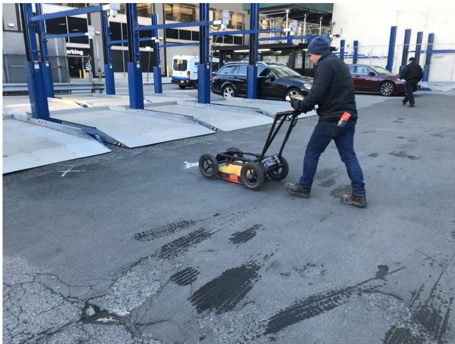
Photo 1, 4/20/2018: View of NOVA Geophysical clearing a boring location using ground penetrating radar (GPR) (facing northeast)
