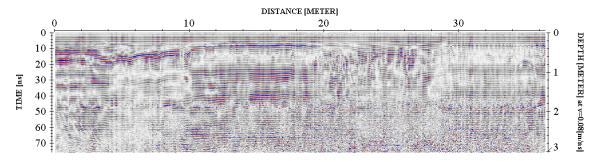
**Step 4.** Remove static from bottom of profile (time cut)
