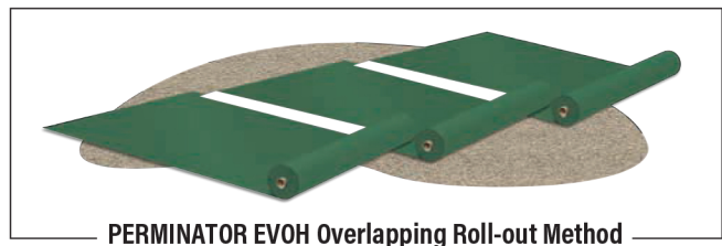
PERMINATOR EVOH Overlapping Roll-out Method
