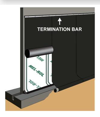
Backfilling should be done immediately, using care and caution to avoid damaging the water-proofing application.
