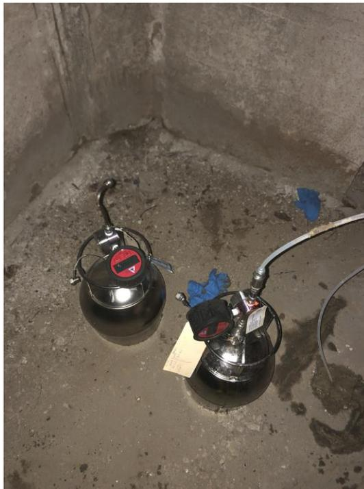
Photo 2: View of sub-slab vapor point and co-located indoor air samples SSV/IA12 (facing north).
