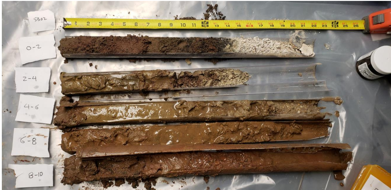
Photo 1, 5/31/2018: Soil recovery from soil boring SB2, facing down.
