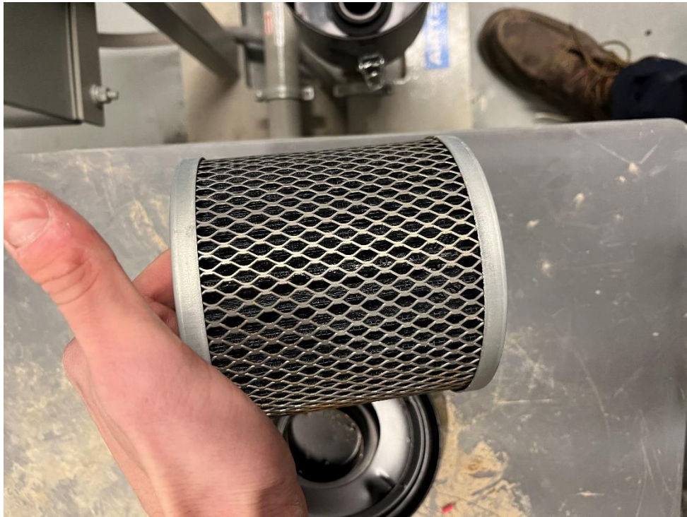
Photo 7, 01/17/2023: View of SMD system blower filter
