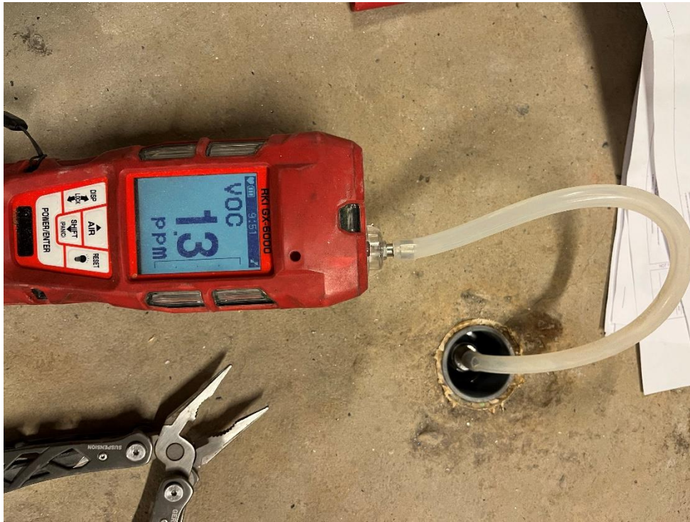
Photo 23, 01/17/2023: Langan collecting PID readings from vapor monitoring point VMP03
