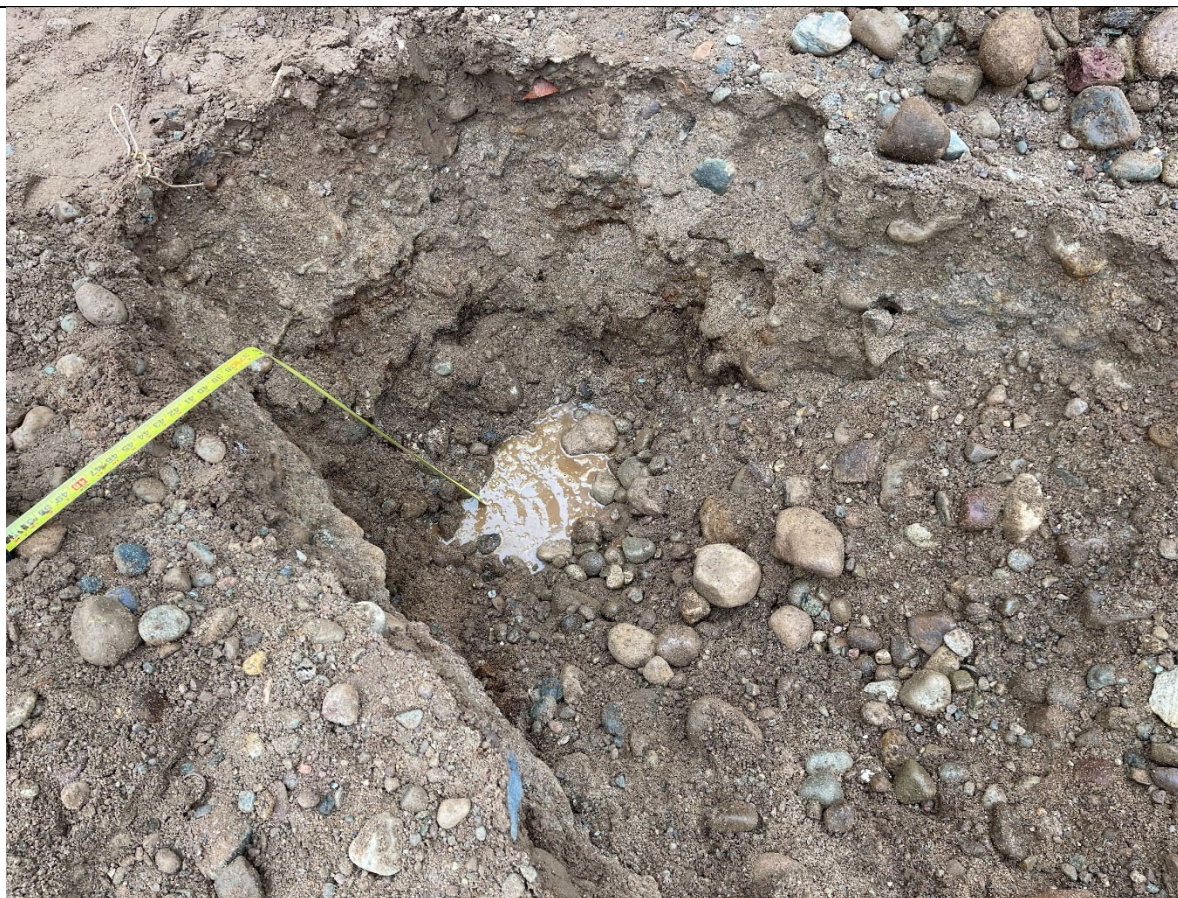
Photo 4 - View of depth to groundwater at 16.5'.
