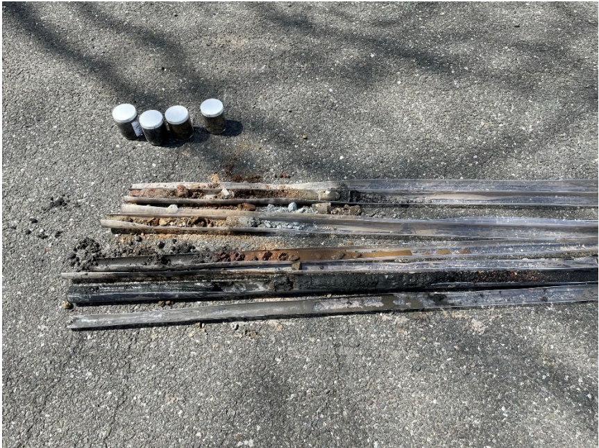
Photo 4: Looking north, sleeves and sampled soil.
