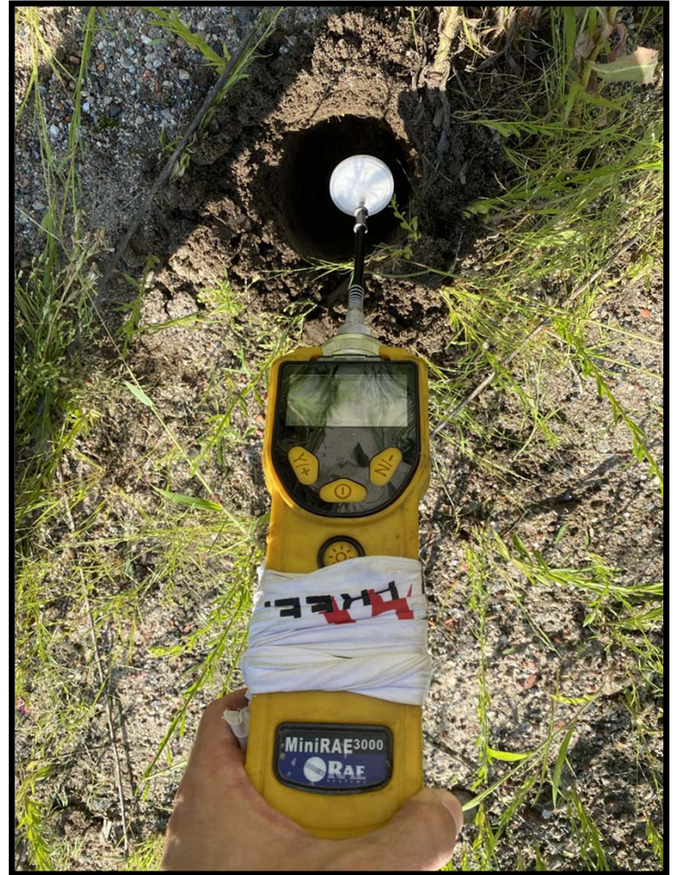
View of a soil boring being screened for VOCs with a PID.
