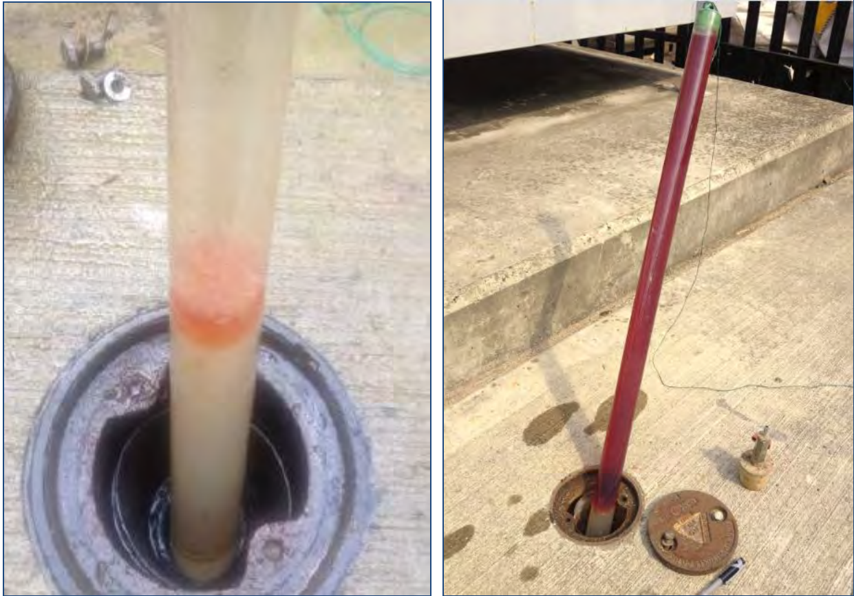
Figures 5a and 5b. Visible separate-phase hydrocarbon pre-PetroCleanze (left) and post-PetroCleanze (right) application. Commercial yard, southern UK.
