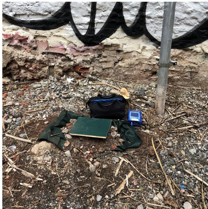
Photo 2: Seismograph placed adjacent to the 110 Greenwich Street building during caisson drilling work, looking east.
