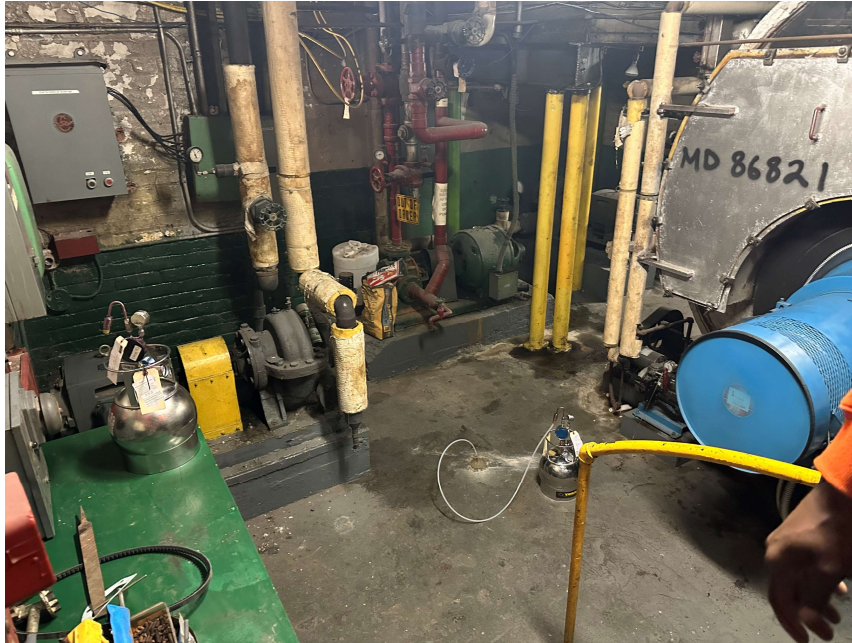
Sub-slab vapor and indoor air sampling
