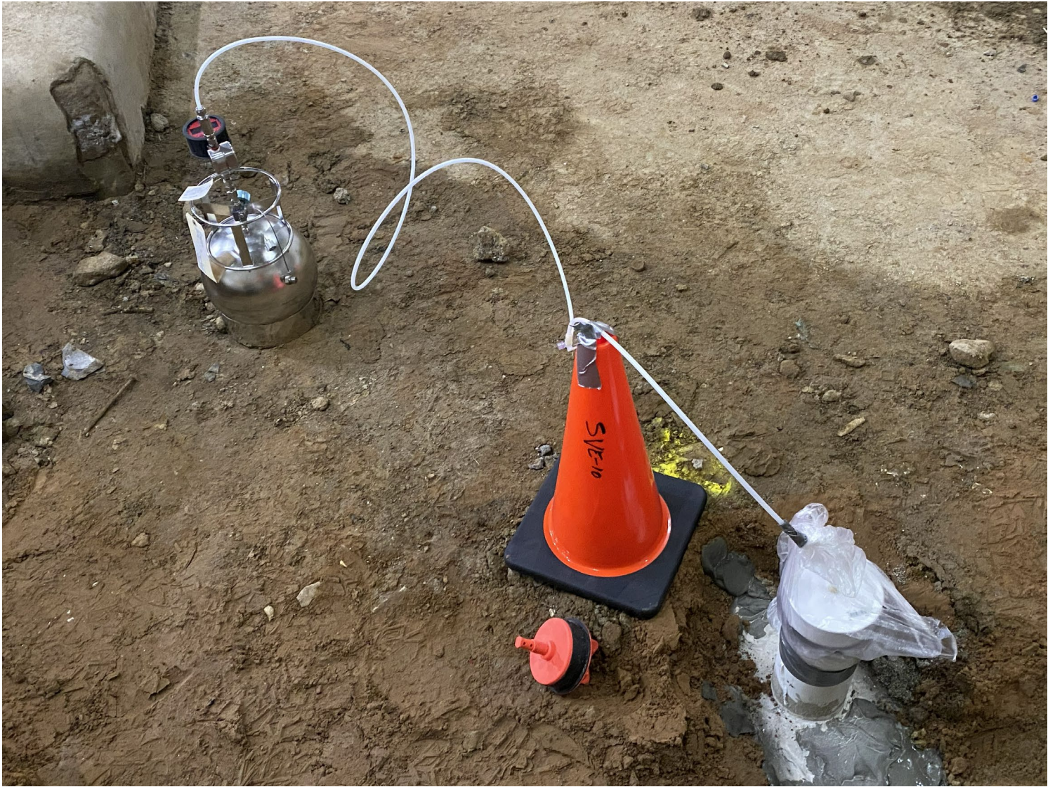
Photo 3: 24 Hour Summa Canister Set Up For SVE-10
