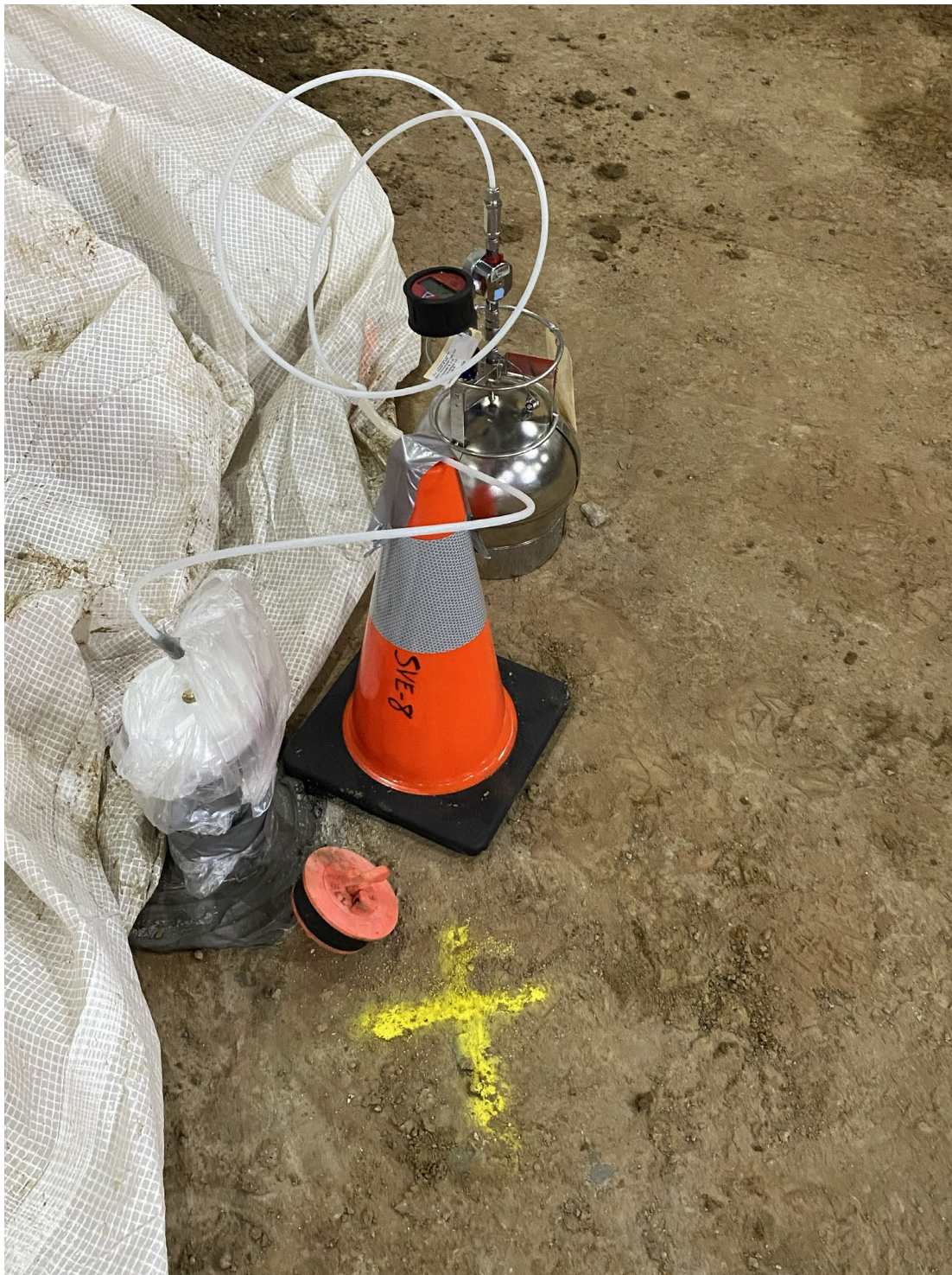
Photo 1: 24 Hour Summa Canister Set Up For SVE-8
