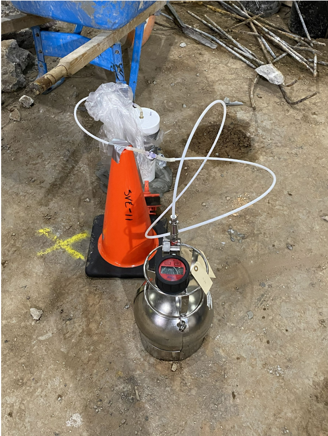
Photo 4: 24 Hour Summa Canister Set Up For SVE-11
