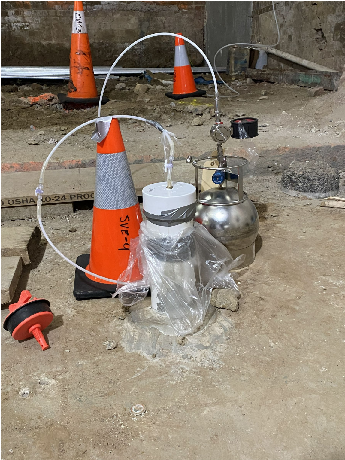
Photo 2: 24 Hour Summa Canister Set Up For SVE-9
