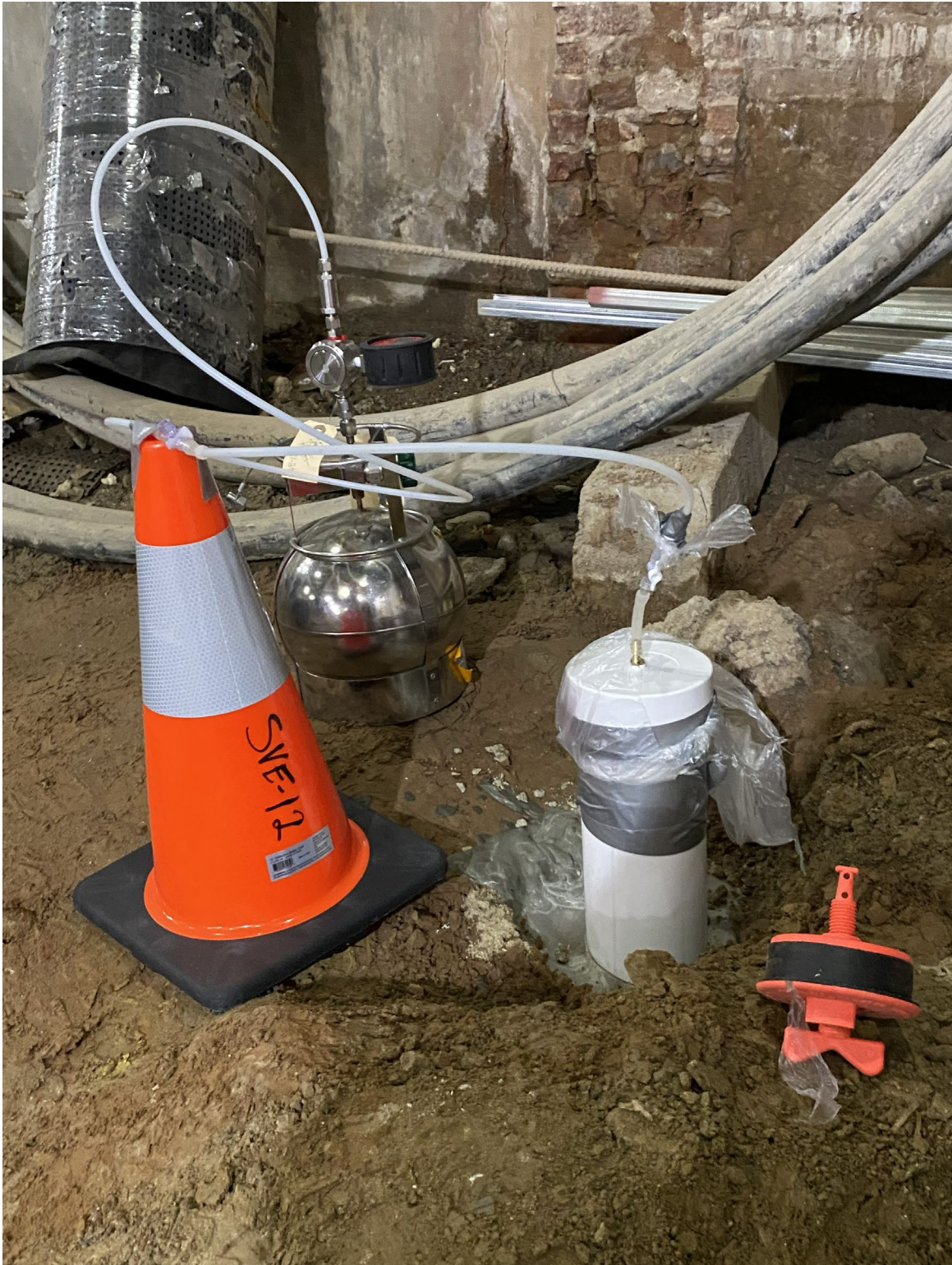
Photo 5: 24 Hour Summa Canister Set Up For SVE-12
