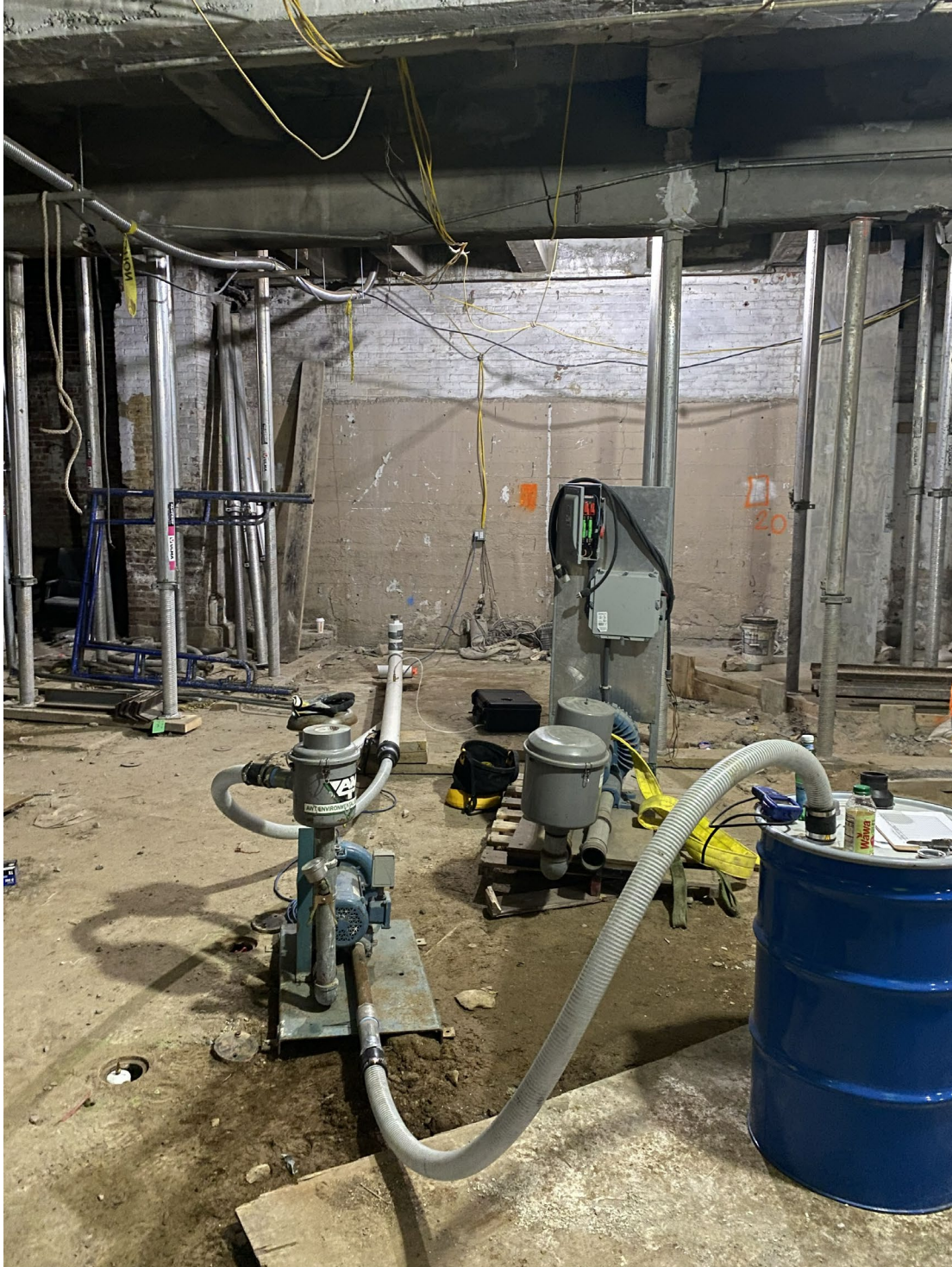
Photo 1: Pilot test on SVE-3, with blue carbon drum
