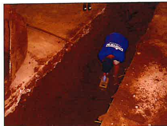
6. Hydrogeologist screening trench in Sample location #3 with a PID.
